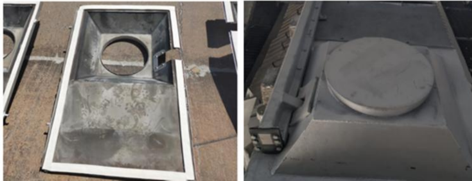
Figure 3. Pot cover gaskets and sealing.
