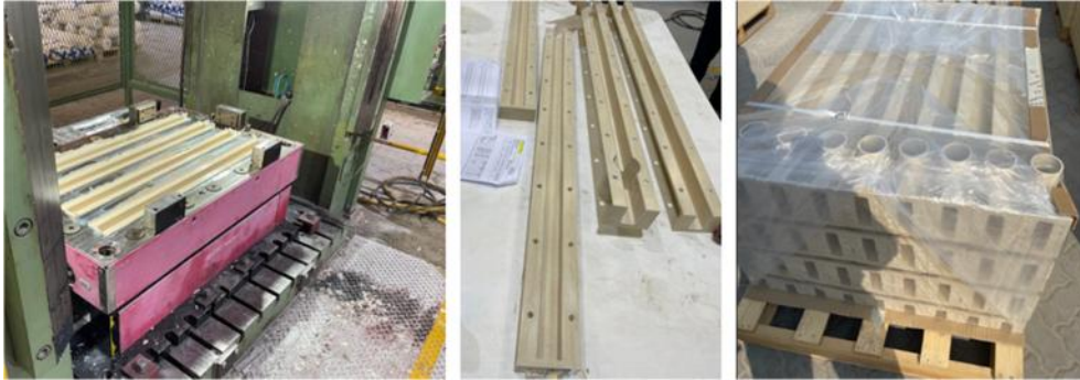
Figure 5. GRP Insulation air slide molding in UAE.
