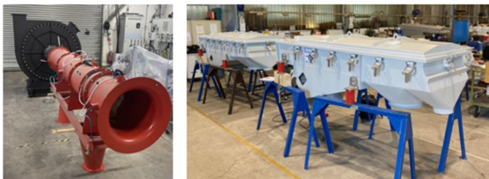
Figure 7. Fluidising fan and vibration sieve testing in UK and Germany
