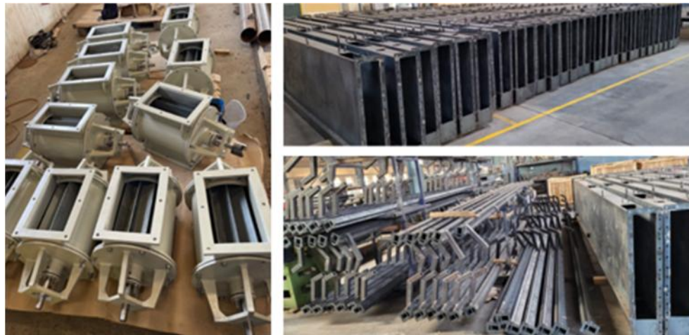
Figure 6. Rotary feeder and air slide fabrication in UAE
